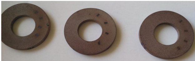
Figure 5. Traces of coating wear after friction tests
